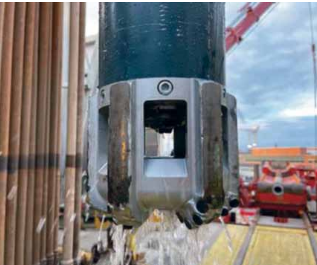
Fig-7 The CoDril™ tool is a supplemental downhole convertible core bit that can switch between coring and drilling modes.
